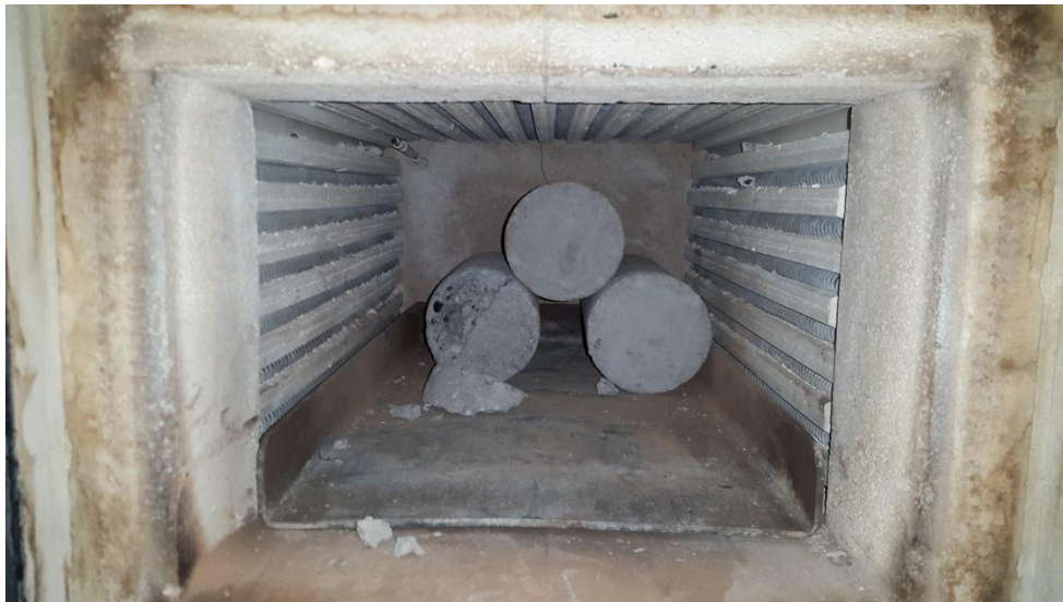
Figure 1: Spaling of cylinder specimens after exposure to 450°C.
