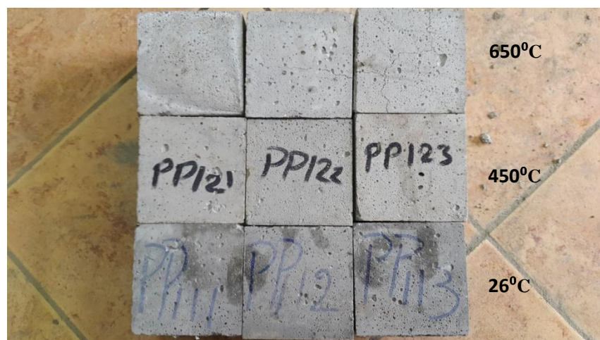
Figure 4: Polypropylene contained cube specimens after exposure to different temperatures
