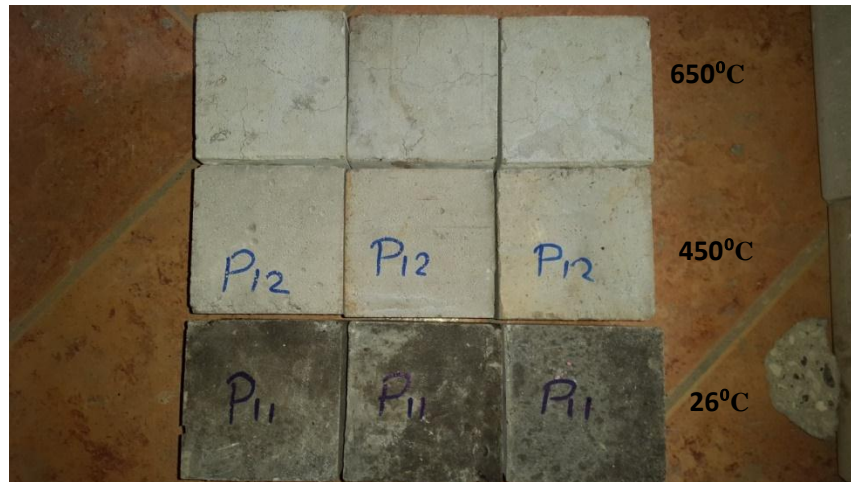
Figure 3: Non-polypropylene contained cube specimens after exposure to different temperatures
