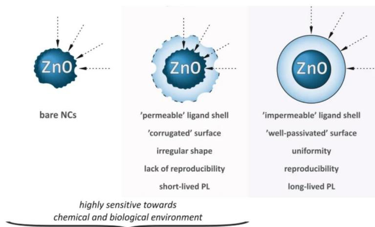
Figure 6: Schematic representation of nanocrystal-ligand interface structure of ZnO NPs (Wolska-Pietkiewicz et al., 2019)
