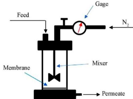
Figure 7: Schematic diagram of the filtration system (Kakar et al., 2022)
