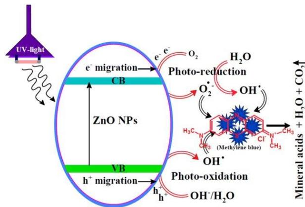
Figure 2: Schematic representation of photocatalytic degradation using ZnO nanoparticles (Alshehri & Malik, 2019)
