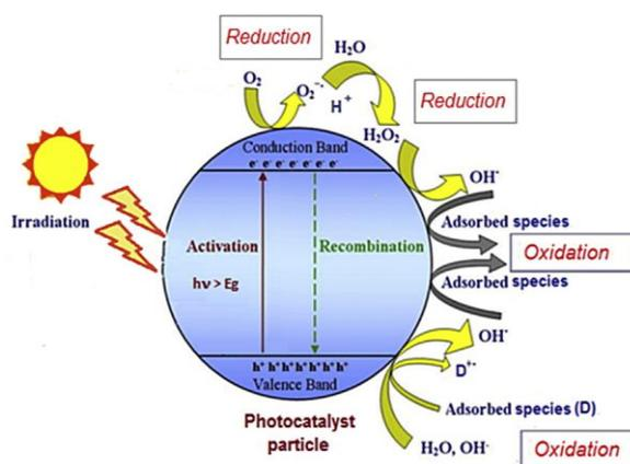
Figure 3: Heterogeneous photocatalytic oxidation steps (Spasiano, Marotta, Malato, Fernandez-Ibanez, & Di Somma, 2015)
