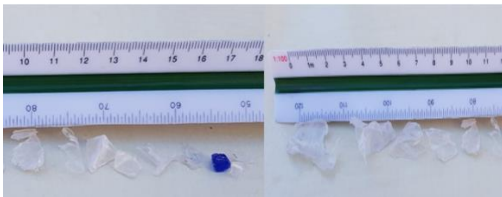
Figure 1: Plastic waste as fine and coarse aggregate
