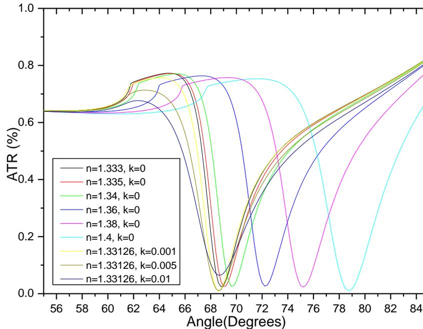
Figure 3: Comparison of the theoretically calculated reflectivity (ATR%) with respect to angle of incident light of different samples with various real and imaginary components
