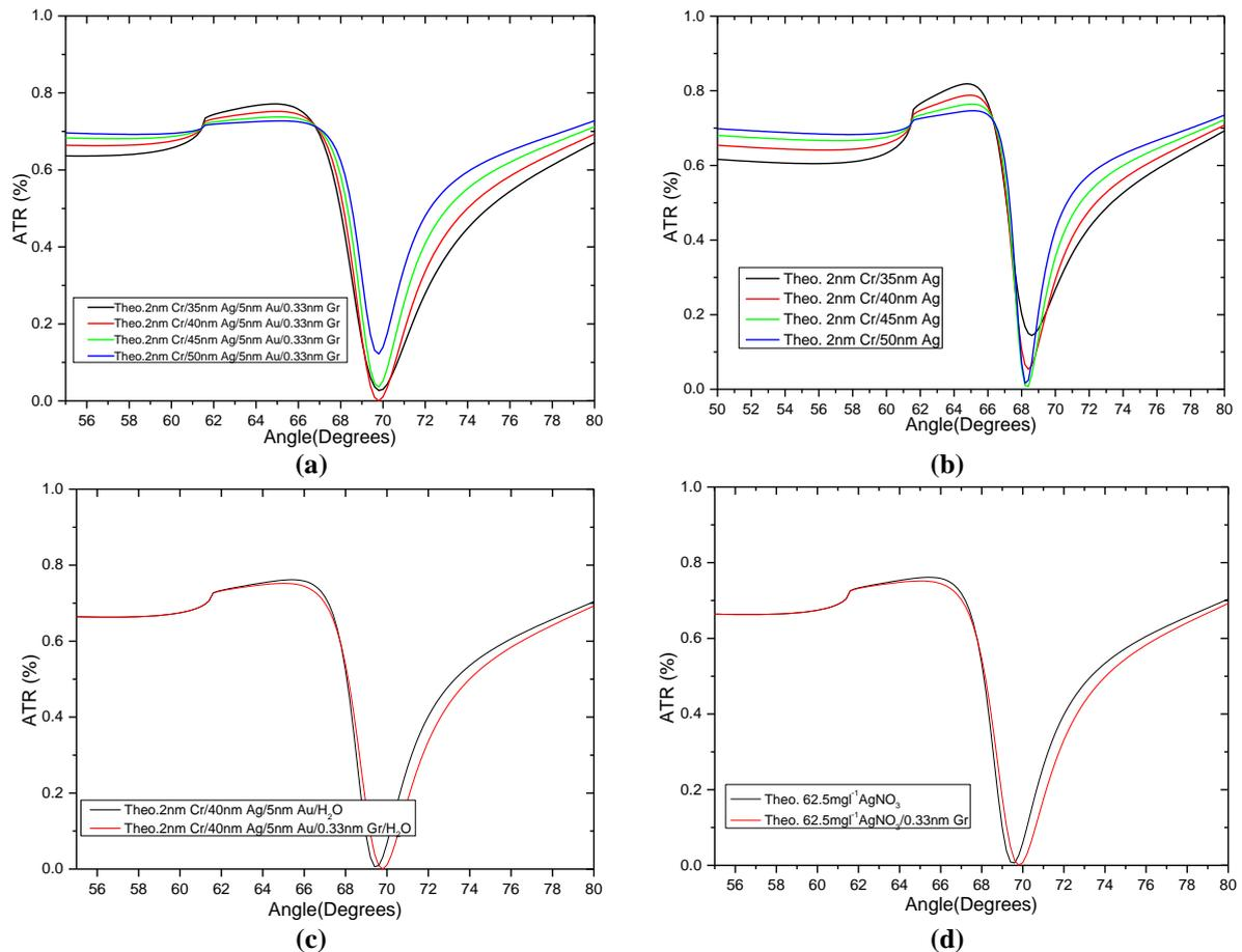
Figure 4: Intensity of reflected light with respect to incidence angle. (a) and (b) SPR reflectivity from silver layers with different thicknesses in the presence and absence of a 5 nm-thick protective gold or graphene layer. (c) and (d) Comparison between the SPR results of a multi-layered system with a graphene layer, those of a pure water system and those of a  $\text{AgNO}_3$  solution system that lacks imaginary components
