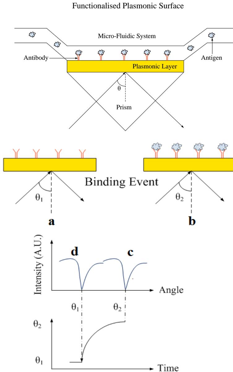
Figure 1: SPR immunoassay technique. (a) and (b) Antibody-functionalised SPR sensor layer on the top of a conventional glass prism/gold plasmonic system. (c) Angles  $\theta_1$  and  $\theta_2$  before and after the binding event. (d) Change in sensogram following the binding event (Salah, Jenkins, & Handy, 2014).
