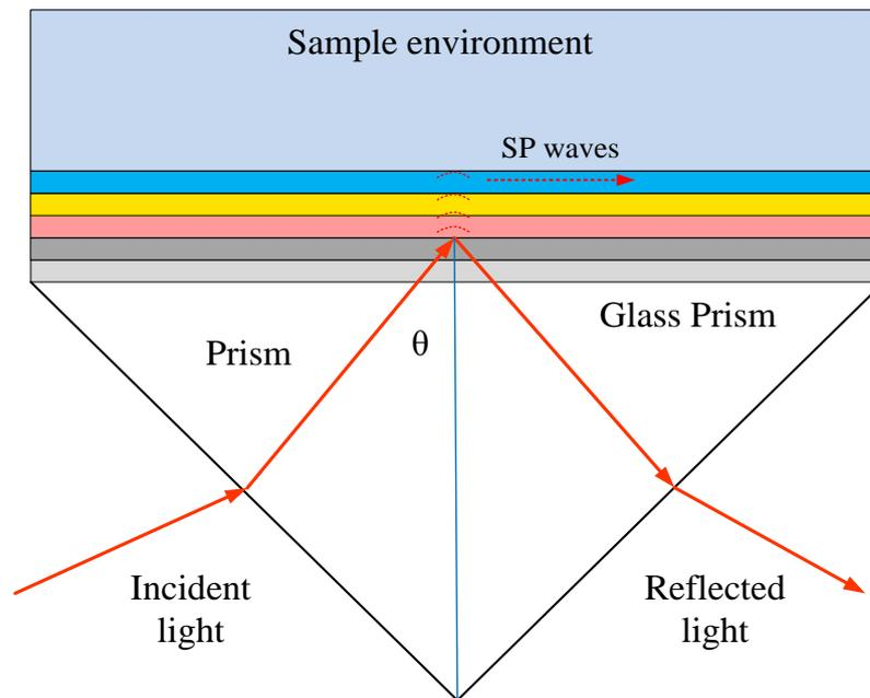
Figure 2: Kretschmann configuration set-up comprising a glass prism, glass substrates and plasmonic layers (Tudos, 2008). The dielectric sample is placed on the top of the set-up. Incident light is refracted towards plasmonic layers at an incidence angle. The evanescent SP wave dominates at the plasmonic–sample environment interface
