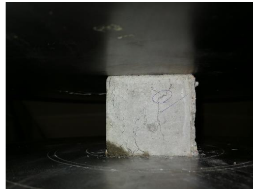
6b. 10% wood fiber/cement specimen
