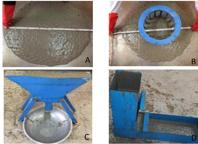
Figure 3: Rheological properties tests: a- slump flow, b- j-ring , c- V-funnel, d- L-box
