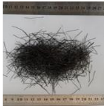
Figure 2: Sample of the recycled steel fibers used in current study (for fibers with length =35mm)
