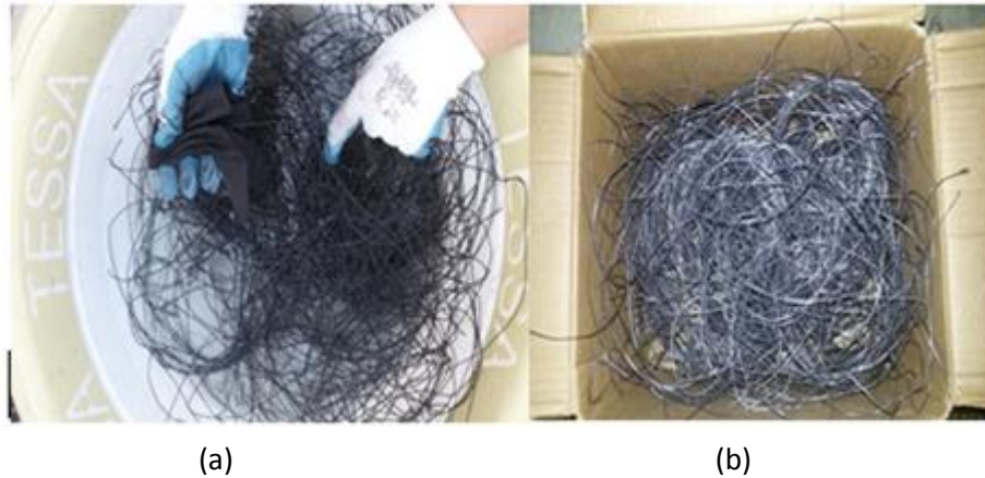
Figure 1: Recycled steel wires a-before cleaning, b- after cleaning
