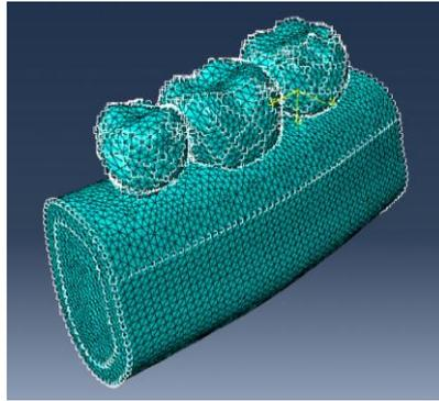
Figure 2. The developed finite element model of the implant supported fixed partial denture
