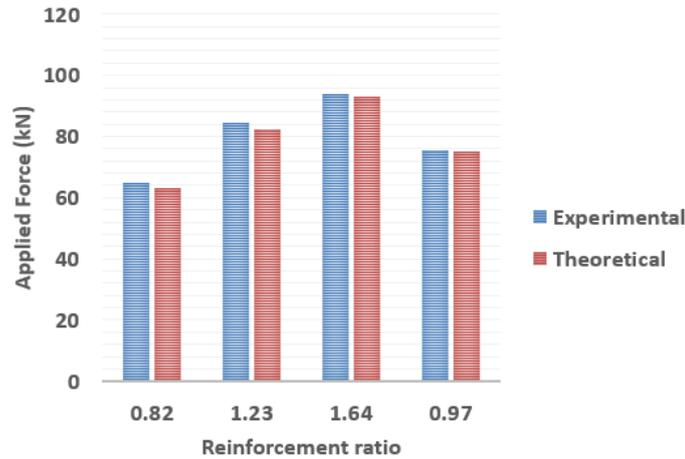
Figure 13: Analytical and experimental beam capacity vs Reinforcement Ratio for G2- $f_c=80$ MPa
