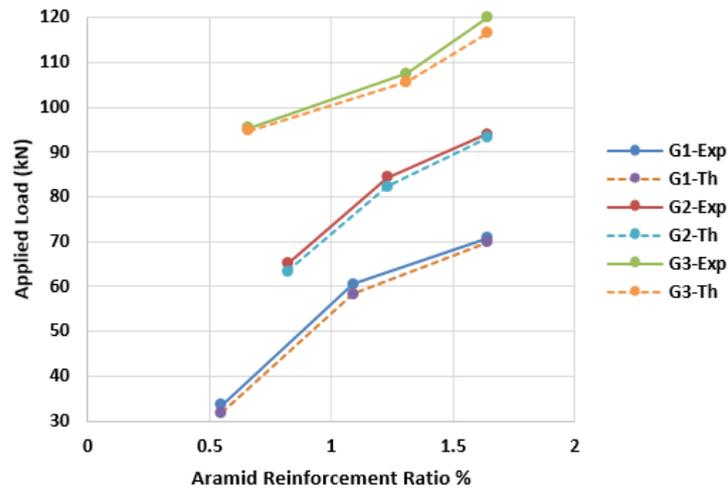
Figure 11: Analytical and experimental beam capacity vs Reinforcement Ratio
