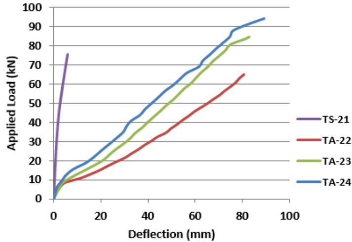
Figure 6: Force-Displacement response for G2-  $f_c = 80\text{MPa}$  Aramid and steel reinforced T-beams
