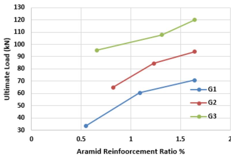
Figure 4: Ultimate load capacity vs AFRP ratio
