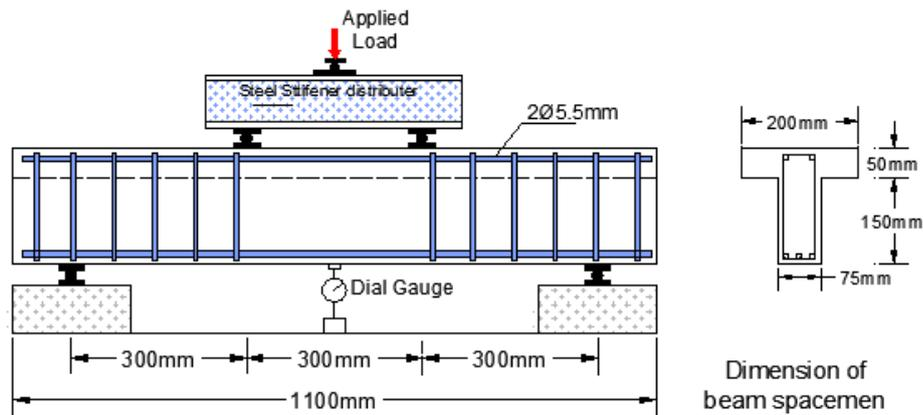
Figure 1: Tested beam geometry
