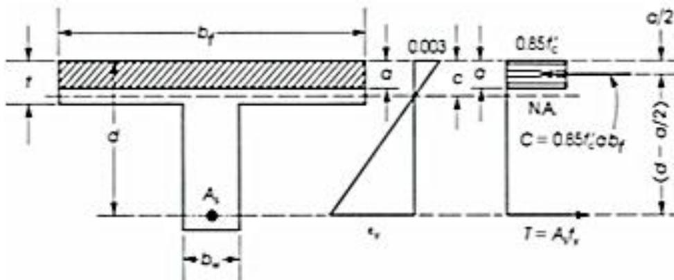
Figure 9: Flanged T-beam ( $a \leq h_f$ )
