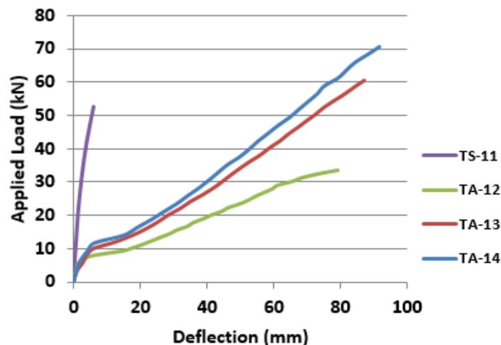
Figure 5: Force-Displacement response for G1-  $\hat{f}_c = 60\text{MPa}$  Aramid and steel reinforced T-beams
