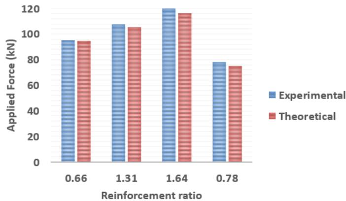
Figure 14: Analytical and experimental beam capacity vs Reinforcement Ratio for G3- $f_c=100$ MPa
