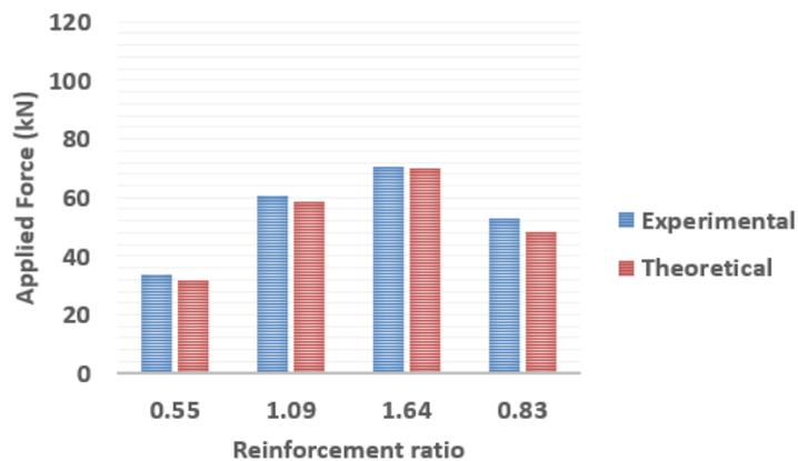
Figure 12: Analytical and experimental beam capacity vs Reinforcement Ratio for G1- $f'_c=60\text{MPa}$
