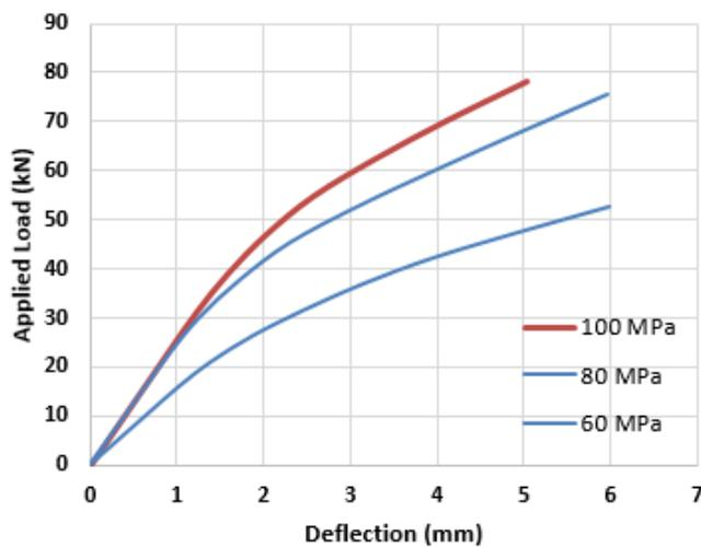
Figure 8: Force-Displacement response for steel reinforced T-beams
