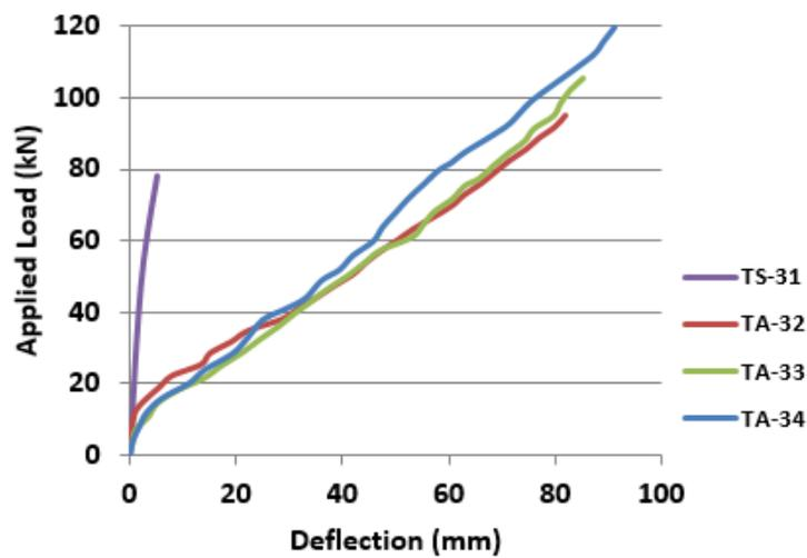
Figure 7: Force-Displacement response for G3-  $f_c = 100\text{MPa}$  Aramid and steel reinforced T-beams
