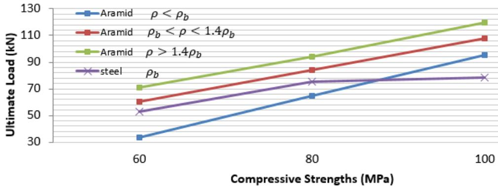
Figure 3: Ultimate load capacity vs SCC strength
