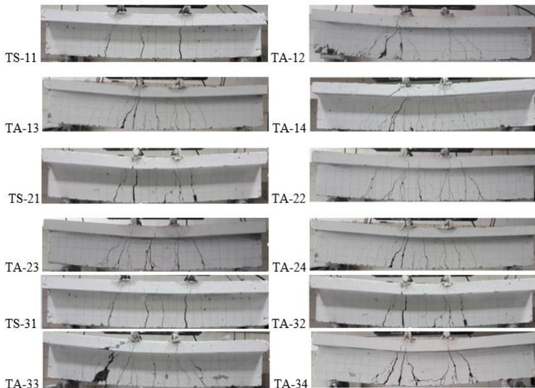
Figure 2: Crack pattern of T-beams
