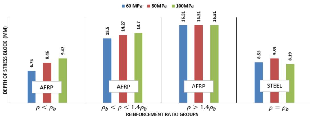
Figure 10: Effect of SCC compressive Strength on Equivalent stress block
