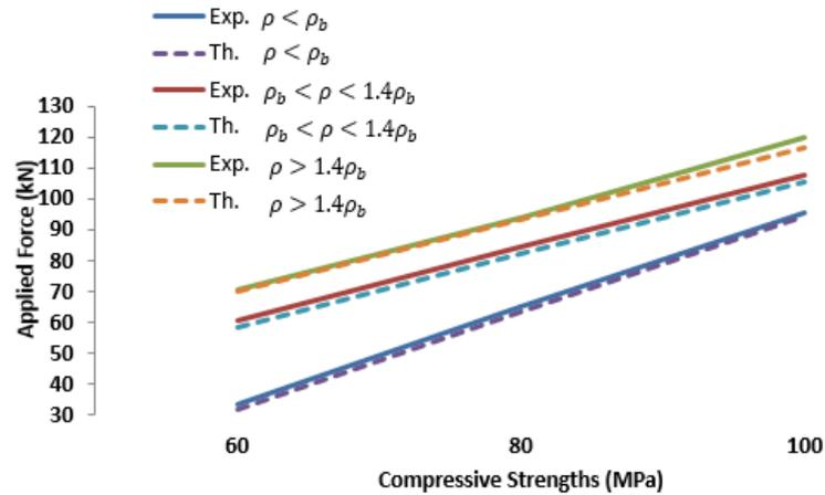
Figure 10: Analytical and experimental beam capacity vs SCC strength
