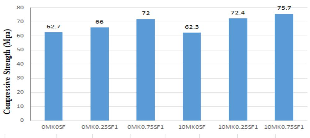
Figure 3: Effect of steel fiber and MK incorporated concretes on the compressive strength
