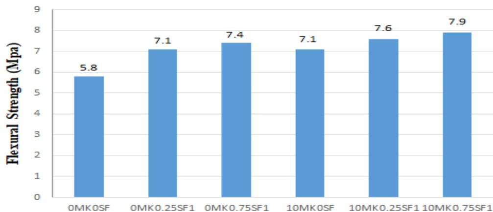
Figure 4: Effect of steel fiber and MK incorporated concretes on the three-point flexural strength
