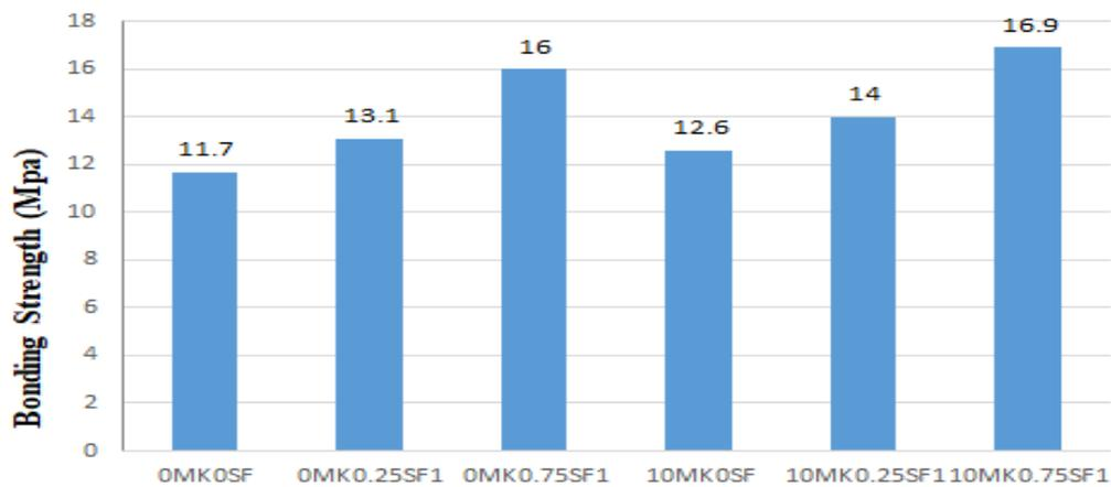
Figure 5: Effect of steelfiber and MK incorporated concretes on the bond strength
