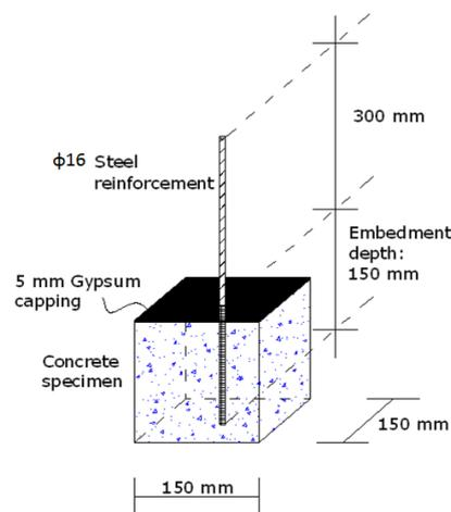
Figure 2: Details of the bonding strength examined samples
