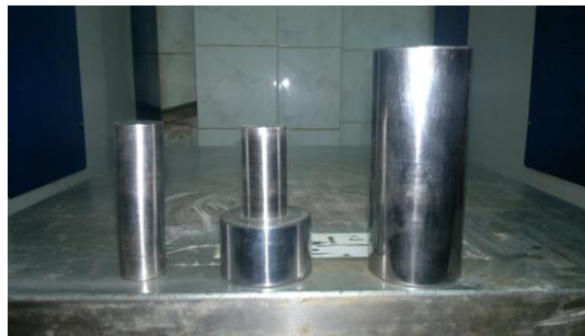
Figure 4: Die assemble for produce a composite powder compact the rough shape particles of Al 2 O 3 powder (100 mesh)
