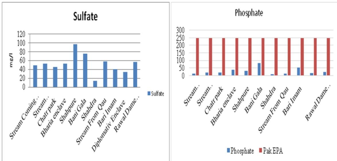
Figure 4: Water sample analysis for sulphate and phosphate
