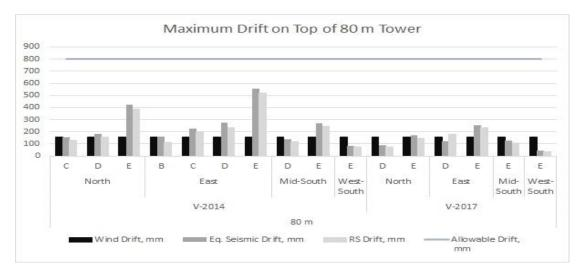
Figure 7: Maximum drift – 80 m tower
