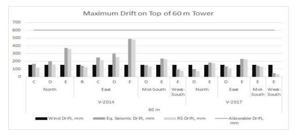
Figure 6: Maximum drift – 60 m tower
