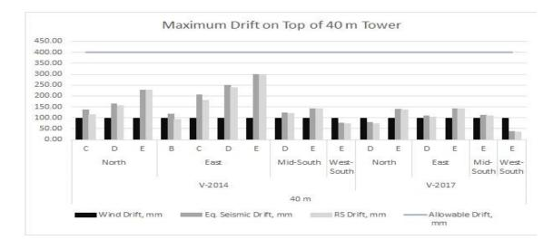
Figure 5: Maximum drift – 40 m tower
