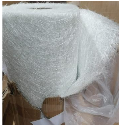
Figure 3: Surface texture of the used GFRP sheets (CSM)
