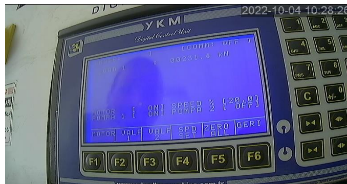
Figure 7: Digital control unit for testing deep beams
