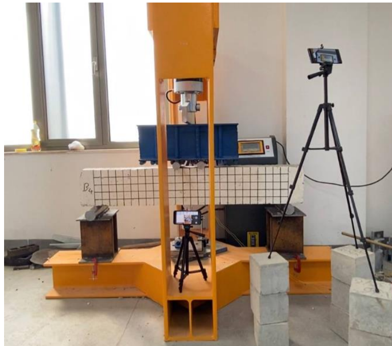
Figure 5: Test setup with the loading frame
