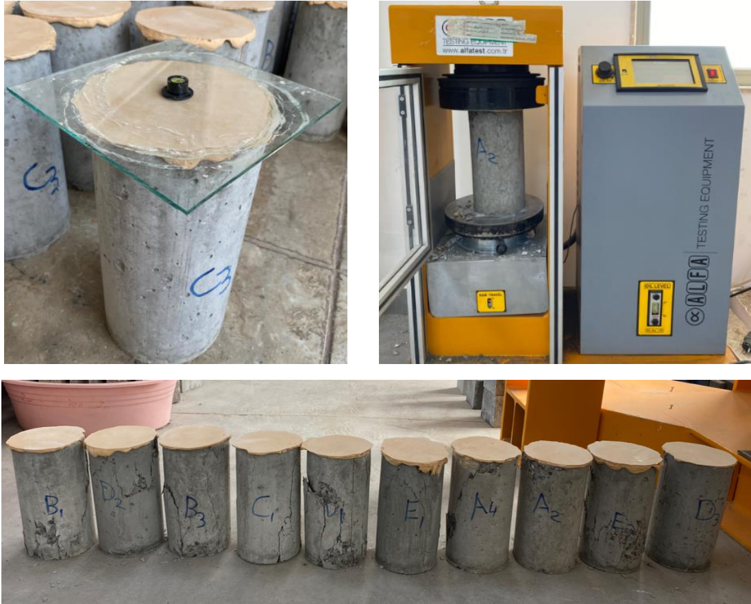
Figure 6: Cylinder capping concrete and compressive testing equipment
