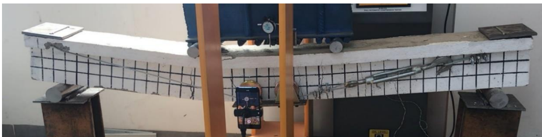
Figure 6: Beam GA1 after failure small crush in compression zone due to bearing
