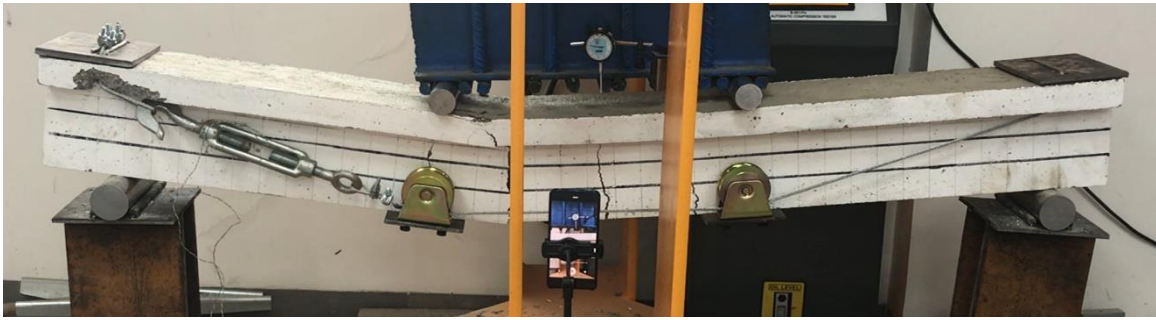
Figure 7: Beam GA2 after failure small crush in compression zone due to bearing
