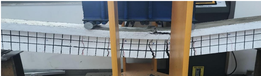
Figure: 5 Control beam crushing at midspan due to compression
