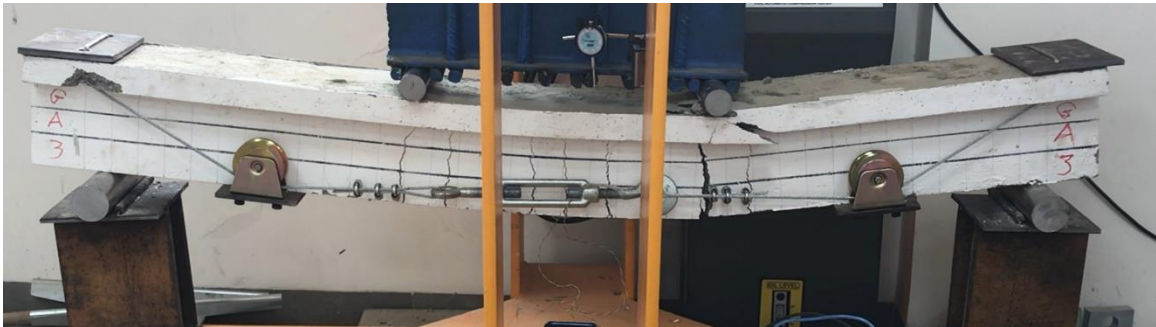
Figure 8: Beam GA3 after failure, crush in compression zone due to bearing
