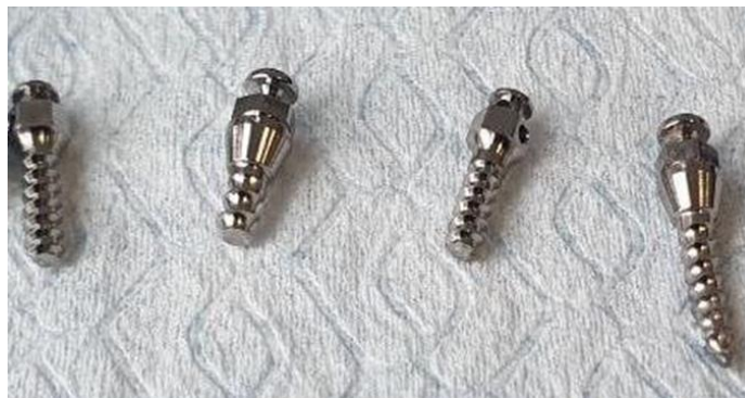
Figure 7: Orthodontic mini-Implants, with different level of fracture.
