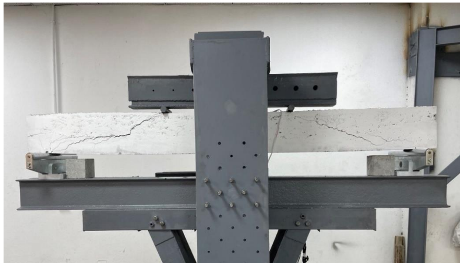
Figure 5: Typical shear failure of an experimental beam.
