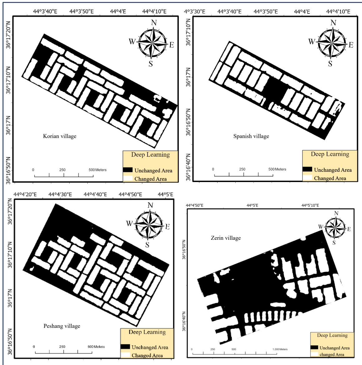
Figure 5: illustrates the building change detection results produced by the deep learning model. The predicted change maps have well-defined building footprints, low levels of noise, and a high degree of spatial coherence in all four study areas. Large residential complexes and smaller individual buildings are outlined with accuracy and are very close to the spatial patterns that exist in the reference maps.
