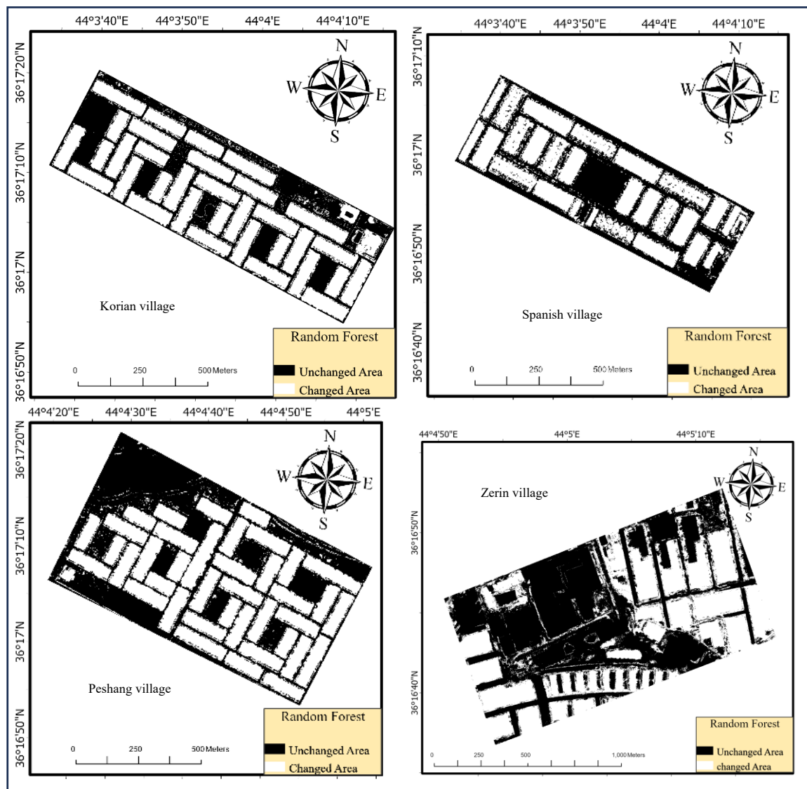
Figure 6: shows the change detection results generated using the Random Forest classifier. Compared to the outputs of the deep learning models, the resulting maps are characterized by an increased level of salt-and-pepper noise, reduced fidelity of building edges, and a higher number of false positives, in particular, in spectrally richer or shadowed areas.
