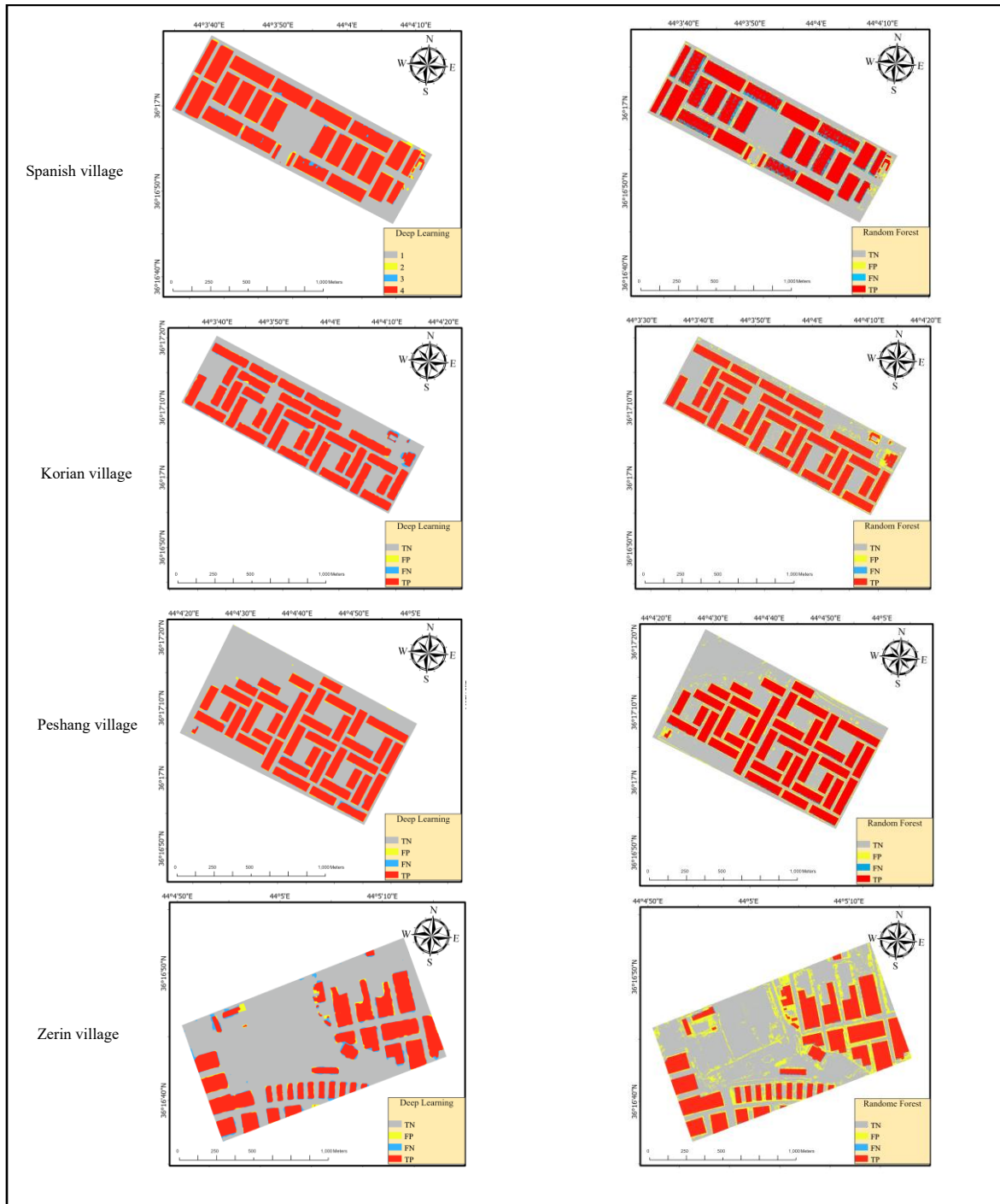
Figure 7: Error maps for deep learning (left) and Random Forest (right) across the study areas, showing true positives (TP), true negatives (TN), false positives (FP), and false negatives (FN).
