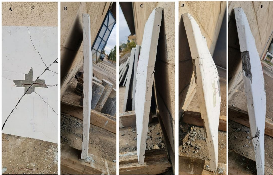
Figure 21: Extent of midpoint deflection of GFE samples with A. 0 layers, B. 2 layers, C. 4 layers, D. 6 layers and E. 8 layers of wire-mesh
