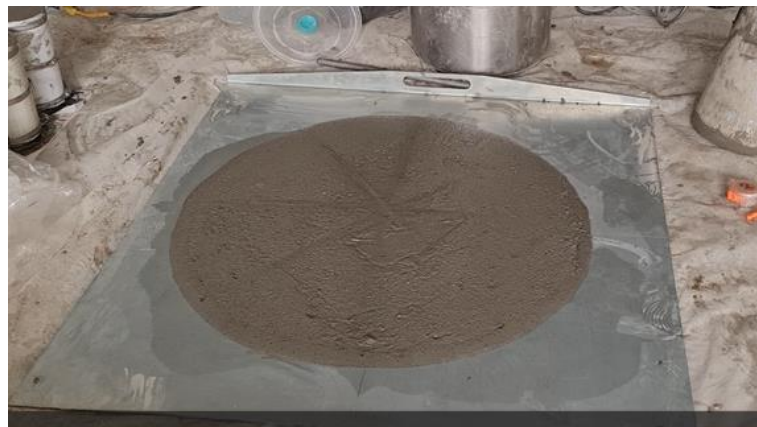
Figure 13: Slump test for the geopolymer mortar
