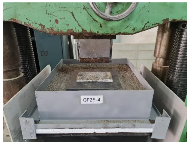
Figure 12: Uniform distribution of load by sand layer
