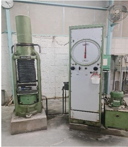
Figure 9: Amsler hydraulic compression machine with capacity of 2000 kN
