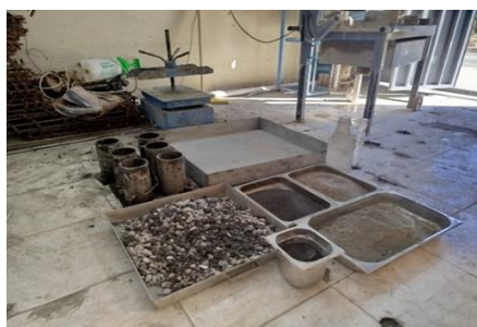
Figure 5: Concrete Materials and Specimen Casting Equipment.
