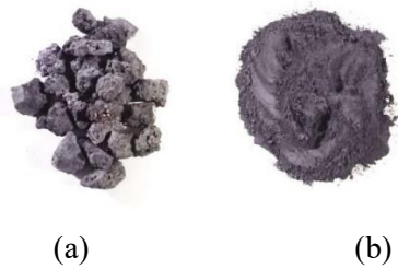
Figure 1: (a) Steel Slag before crushing , (b) Steel Slag after crushing
