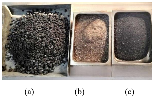
Figure 2: (a) Steel Slag as Gravel (max. size 19.5mm ), (b) Natural Sand, and (c) Steel Slag as Sand.
