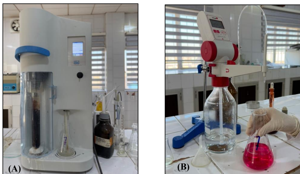
Figure 6: (A) Kjeldahl technique. (B) Titration to determine N%.
