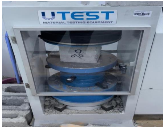
Figure 8: Compressive strength test setup and process
