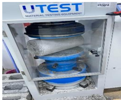
Figure 9: Splitting tensile strength test setup and process
