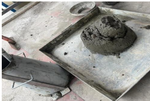
Figure 7: Slump test setup and process
