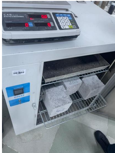
Figure 10: Dry density test setup and process
