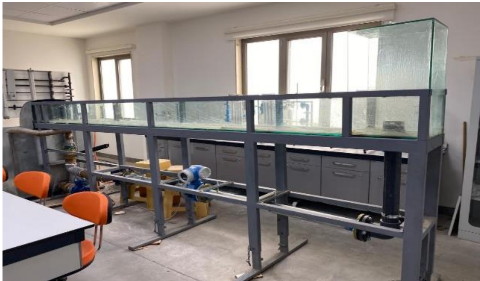
Figure 1: Experimental setup of the open channel in the laboratory
