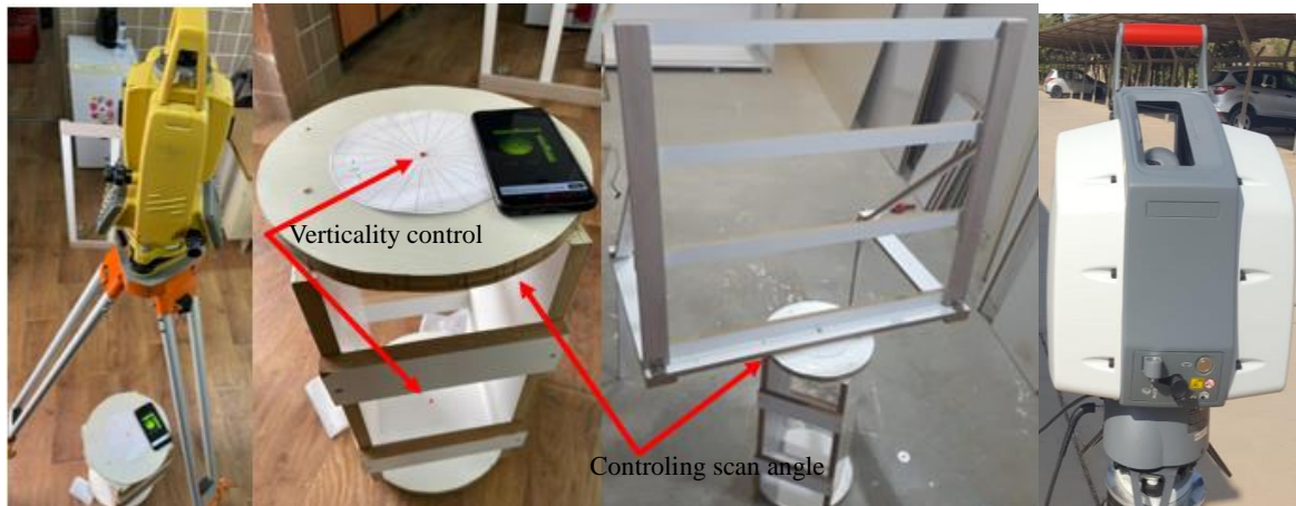
Figure 2: Utilizing the total station instrument's centering vertical laser beam to check the stand's verticality. The left image displays the controlling scan angle, the two right photos represent the verticality test, and the last is the TLS instrument used.
